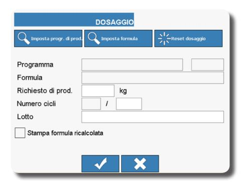
From this screen the operator can select processing through a program or a formula.
